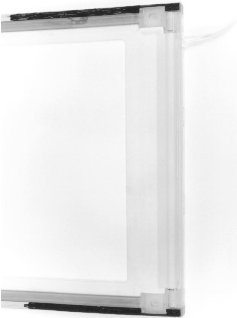
Figure 16. A Custom Designed, Extremely Low Loss Display. All Metal Is Eliminated in Lamp Area (Lower Portion of Photo). A Good Compromise Between Mechanical Strength and Loss Control
