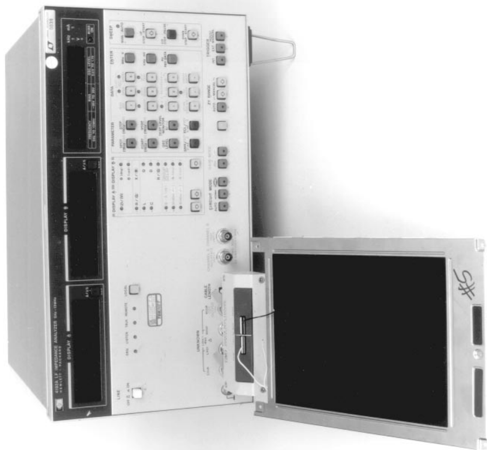
Figure 13. Measuring Lamp Wire to Display Frame Capacitance. Technique Gives Lead Wire-to-Frame Loss Information but Not Lamp-to-Foil -or- Frame Loss Data. Lamp Must Be Energized Before Its Parasitics Are Measurable
